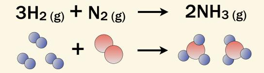
High amounts of NH<sub>3</sub> can be produced at low temperature in presence of a highly active catalytic material<sup>(1)</sup>
